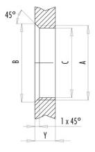
Installation direction: o-ring sits on chamfer.
